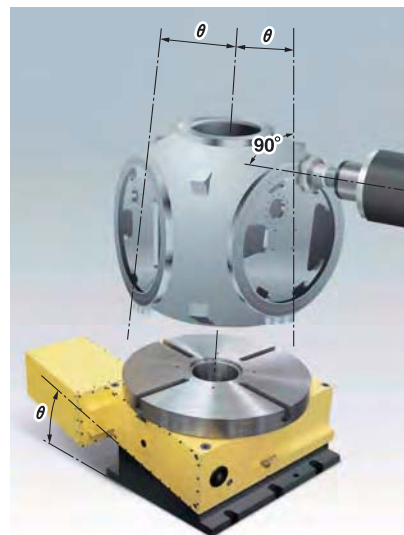
Configuration of the large rotary table on the horizontal M/C to machine a propeller hub of the windmill.
